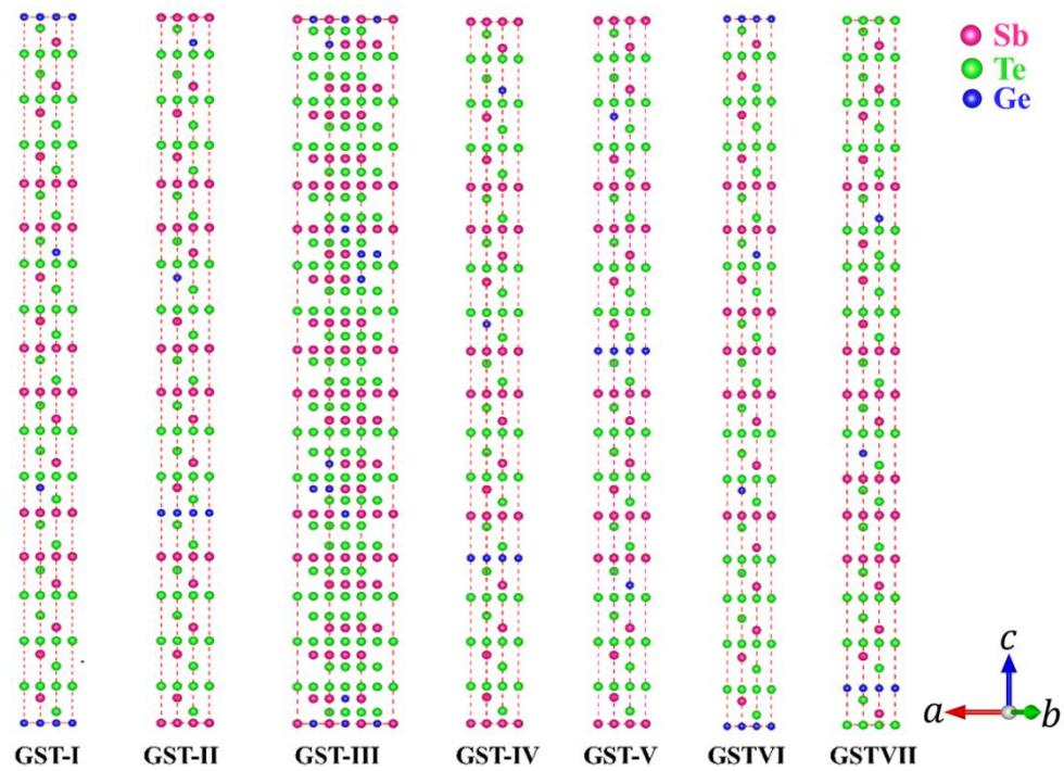
**Supplementary Figure 1.** Hexagonal lattice for seven kinds of atomic stacking configurations of layered  $\text{Ge}_1\text{Sb}_6\text{Te}_{10}$ .
