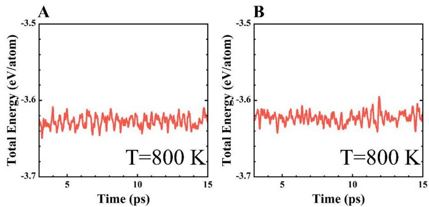
**Supplementary Figure 5.** Evolution of total energy of (A) GST-I and (B) GST-II with respect to time in AIMD simulations at 800 K.
