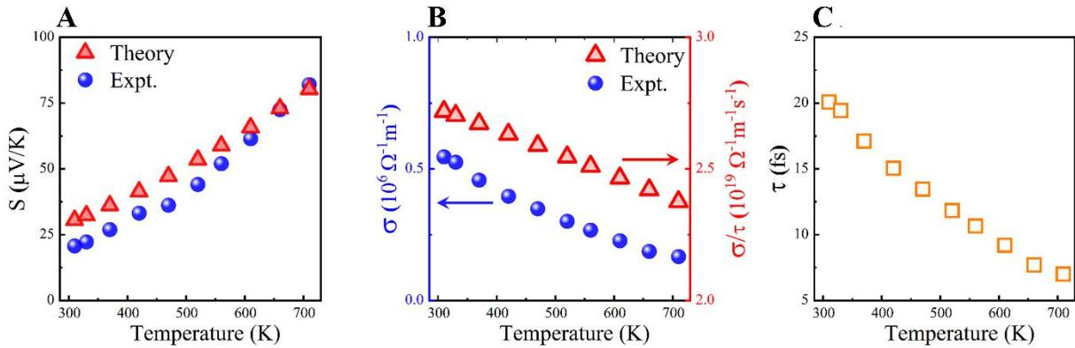
**Supplementary Figure 6.** A: Calculated Seebeck coefficient  $S$  (red triangles) of stacking GST-I at hole concentration of  $7.3 \times 10^{20} \text{ cm}^{-3}$  and available experimental results (blue dots).<sup>[3]</sup> B: Electrical conductivity with respect to relaxation time  $\sigma/\tau$  (red triangles) for stacking GST-I and experimental data of  $\sigma$  (blue dots).<sup>[3]</sup> C: Estimated relaxation time of GST-I at different temperatures.
