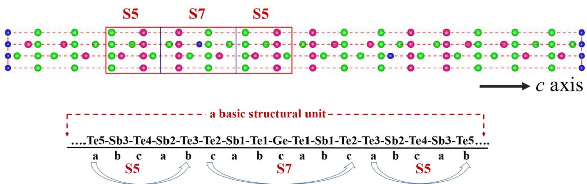
**Supplementary Figure 2.** Crystal structure of atomic stacking GST-I.
