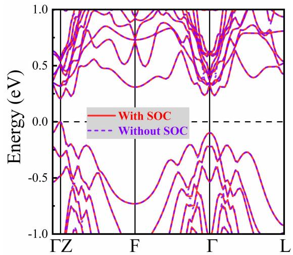
**Supplementary Figure 4.** Electronic band structures of stacking GST-I with and without spin-orbital coupling (SOC).
