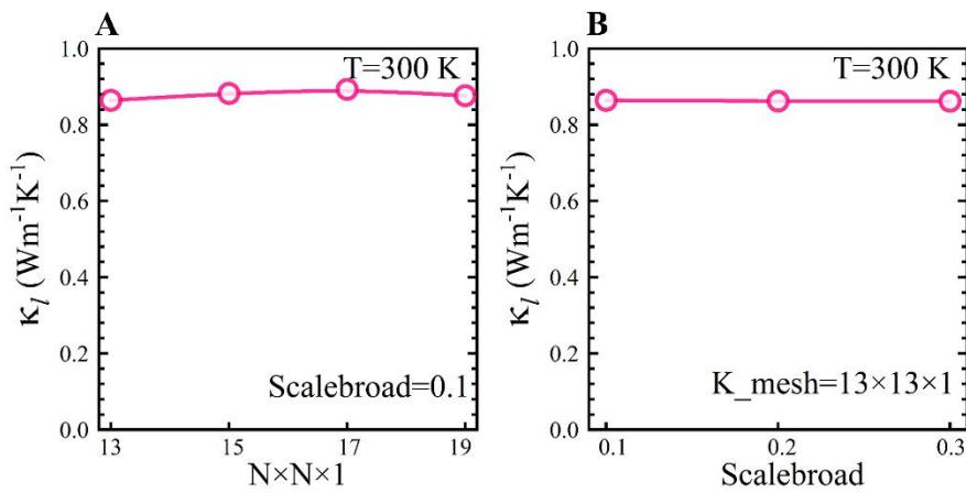
**Supplementary Figure 3.** Convergence tests of lattice thermal conductivity as a function of (A)  $k$ -point grid and (B) scalebroad for stacking GST-I at 300 K.
